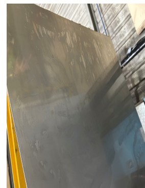
316L slit coil in transport frame | pack edge showing traceability marking and paper staining | staining to unprotected face
