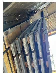
Laser film intact on main faces | typical water staining, exposed face | cases as stored
