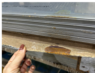
316L slit coil in transport frame | pack edge showing traceability marking and paper staining | staining to unprotected face
