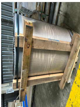
316L slit coil in transport frame | pack edge showing traceability marking and paper staining | staining to unprotected face
