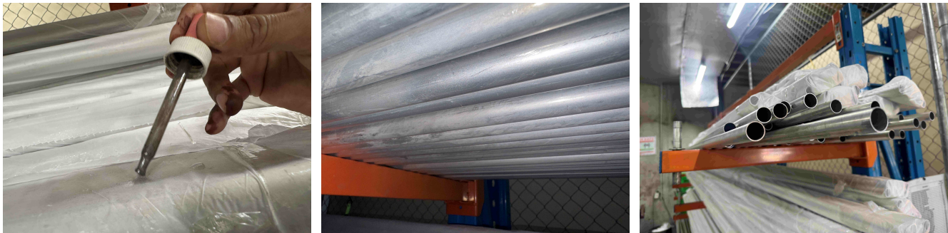
Surface staining detail | bundled stock as racked | open lengths showing bore
