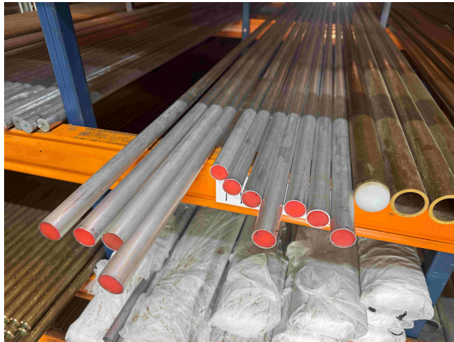
Capped lengths as stored — racked under cover
